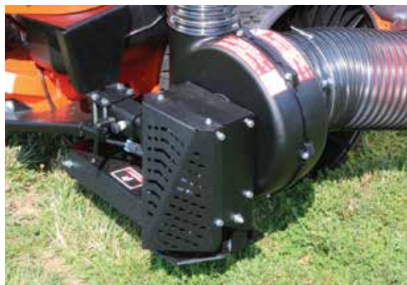
PTO-X Drive System with Self-Tensioning Belt and Electric Clutch Engagement
